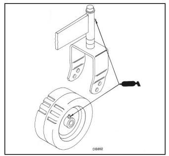
Figure 10. Caster Lubrication
